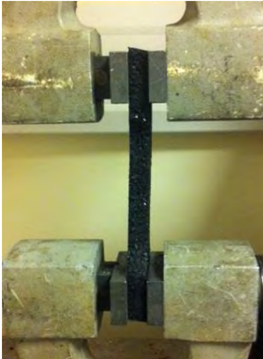
Test piece placed firmly inside the Instron 4411 Tensometer prior to testing. Elongation and load application are set to zero before the test is initiated.
