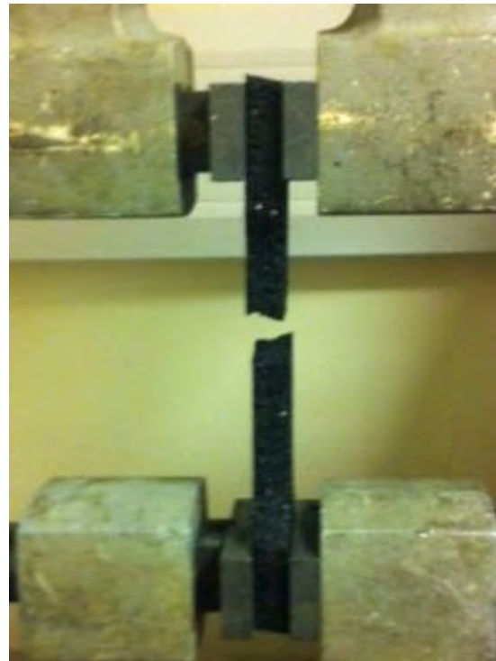
Test piece pulled to destruction, at this point the maximum load applied to the test piece and the maximum elongation are recorded.
