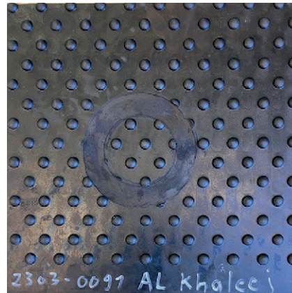
Figure 4: Test sample after abrasion test
